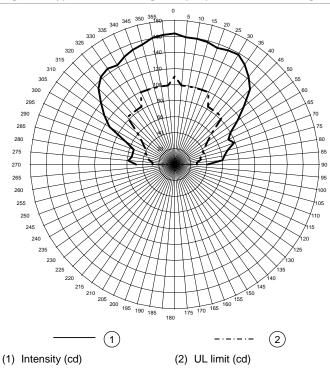
Figure 6: Typical vertical light output profile, 110 cd setting
